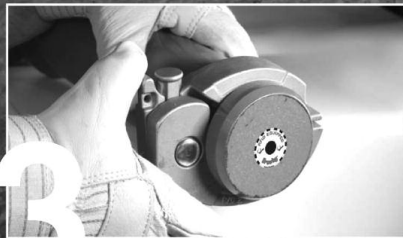
2 Push collar onto bolt
